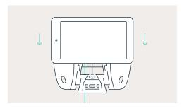
7. Drop the mounting plate cover between the Alarm Panel and wall so that it covers the mounting plate.
