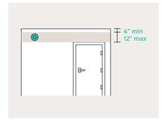
2. Remove the adhesive backing and press the sensor firmly against the mounting surface for 30 seconds to mount the sensor.
