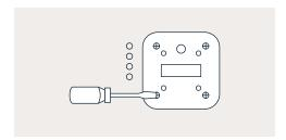
2. Carefully remove the casing and remove the old battery.
