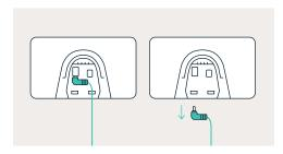
3. Route the power cord through the wire channel on the back of the wall mounting plate.
