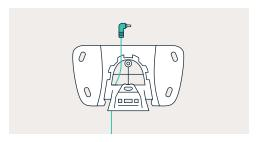
4. Use the included screws and wall anchors to secure the four corners of the mounting plate to the wall.
