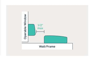
If necessary, place either piece at a 90-degree angle (as long as the pieces are less than one inch apart).
