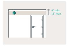
2. Remove the adhesive backing and press the sensor firmly against the
