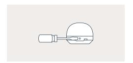
2. Insert your fingernail or a small flathead screwdriver into one of the rectangular pry holes at the bottom of the sensor and pull the case toward you to remove the sensor from the base plate.
