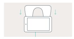
8. Lock the mounting plate cover in place by pressing down on the bottom corners of the cover.
