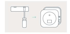
4. Remove the two old AA alkaline batteries.
