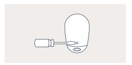
2. Insert a small flathead screwdriver into the small oval opening in the metal key ring while gently twisting. This easily opens the two case halves.
