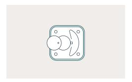
4. Once the new battery is installed, make sure the rubber o-ring is set back in the grooves, which are on the edge of the casing that holds the green circuit board. Then replace the casing, screws, and rubber feet.
