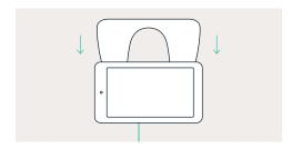
8. Lock the mounting plate cover in place by pressing down on the bottom corners of the cover.
