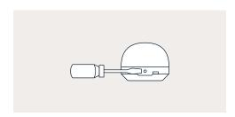
Insert your fingernail or a small flathead screwdriver into one of the rectangular pry holes at the bottom of the sensor and pull the case toward you to remove the sensor from the base plate.
