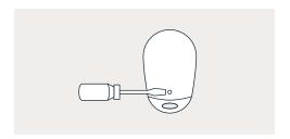
Insert a small flathead screwdriver into the small oval opening in the metal key ring while gently twisting. This easily opens the two case halves.
