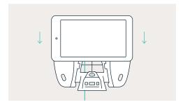
7. Drop the mounting plate cover between the Alarm Panel and wall so that it covers the mounting plate.
