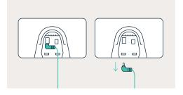
3. Route the power cord through the wire channel on the back of the wall mounting plate.
